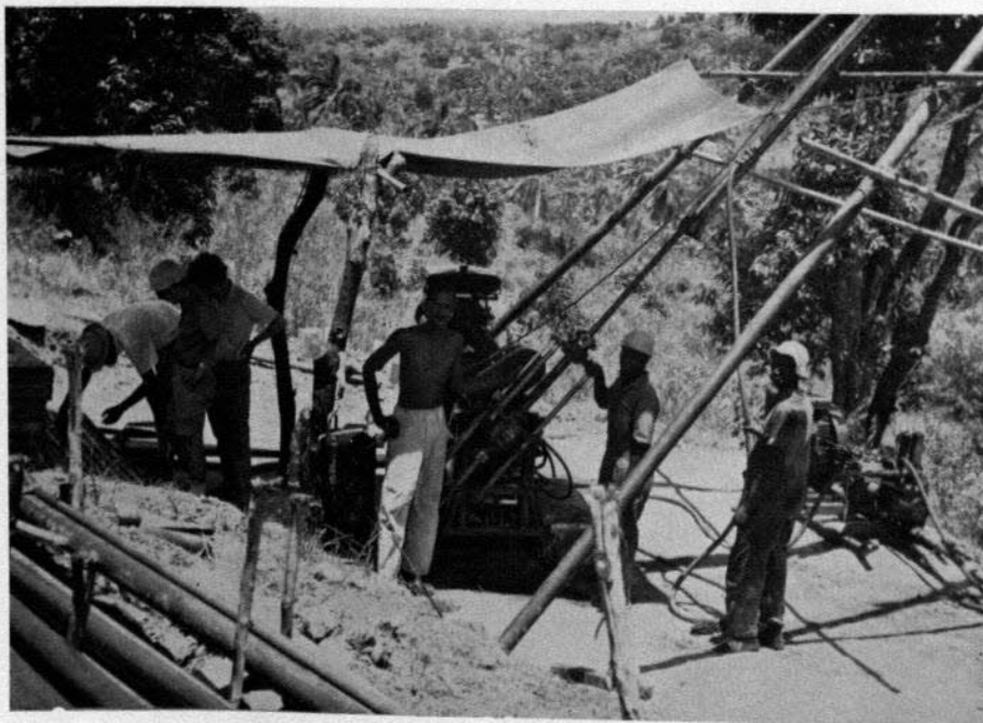
Plate VIIIb—Mines and Geological Department diamond drill working on a lead/zinc prospect near Ribe, Coast Province
