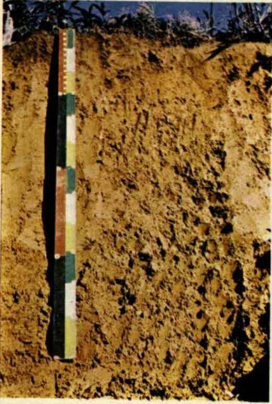
PLATE 1-6 Orthic Acrisol (Tanjong Lipat Family) on sandstone and mudstone at Kiansom. The argillic horizon is deep and stoneless.
