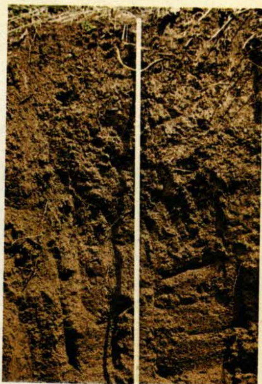
PLATE 1-15 Rhodic Ferralsol (Pinianakan Family) on ultrabasic igneous rocks at Ranau. The oxic horizon is reddish brown and fine-textured.
