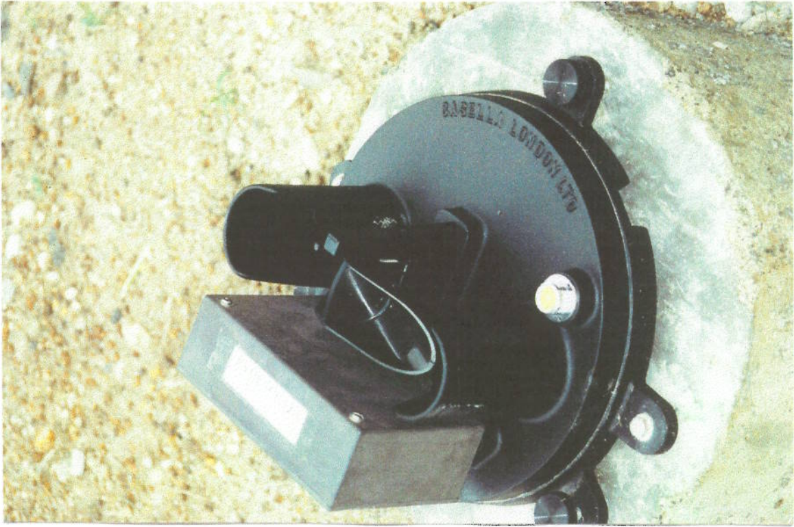
Photo 24 Patience Rainfall Data Logger. Tipping Bucket arrangement.
