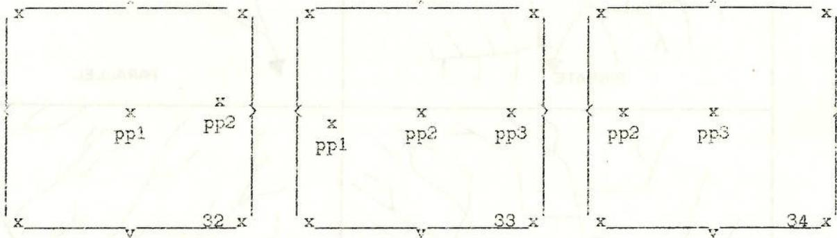
3. Draw flight lines from the principal points through the transferred principal points of the adjacent photos, to the edges of the photos. On the opposite edges of the photos make marks where the flight lines would cross the edges if extended.
