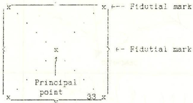
2. Transfer the principal points to the adjacent photos on each side, either by comparing points of detail found on both photos at or near the principal point, or stereoscopically.
